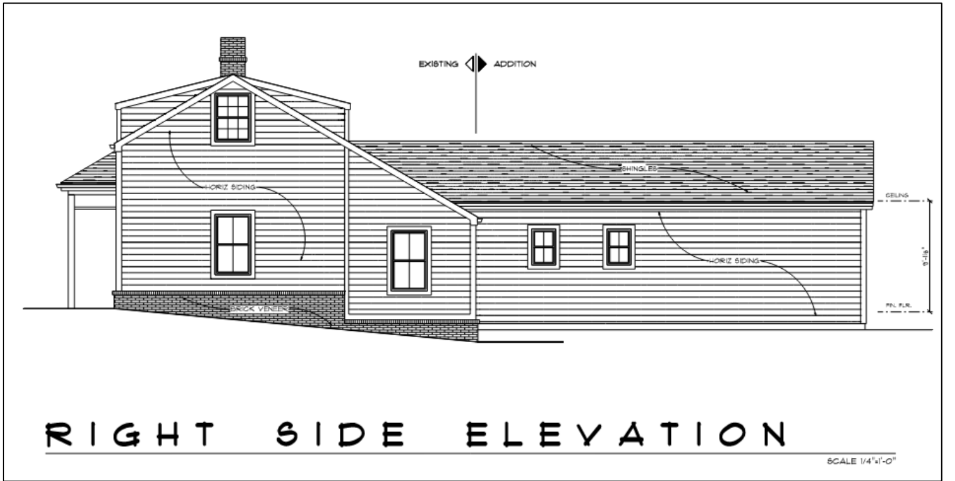
Figure 2: West elevation showcasing addition.
