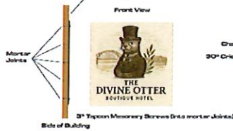
3" Tapered Masonry Screws (into mortar joints) Side of Building
