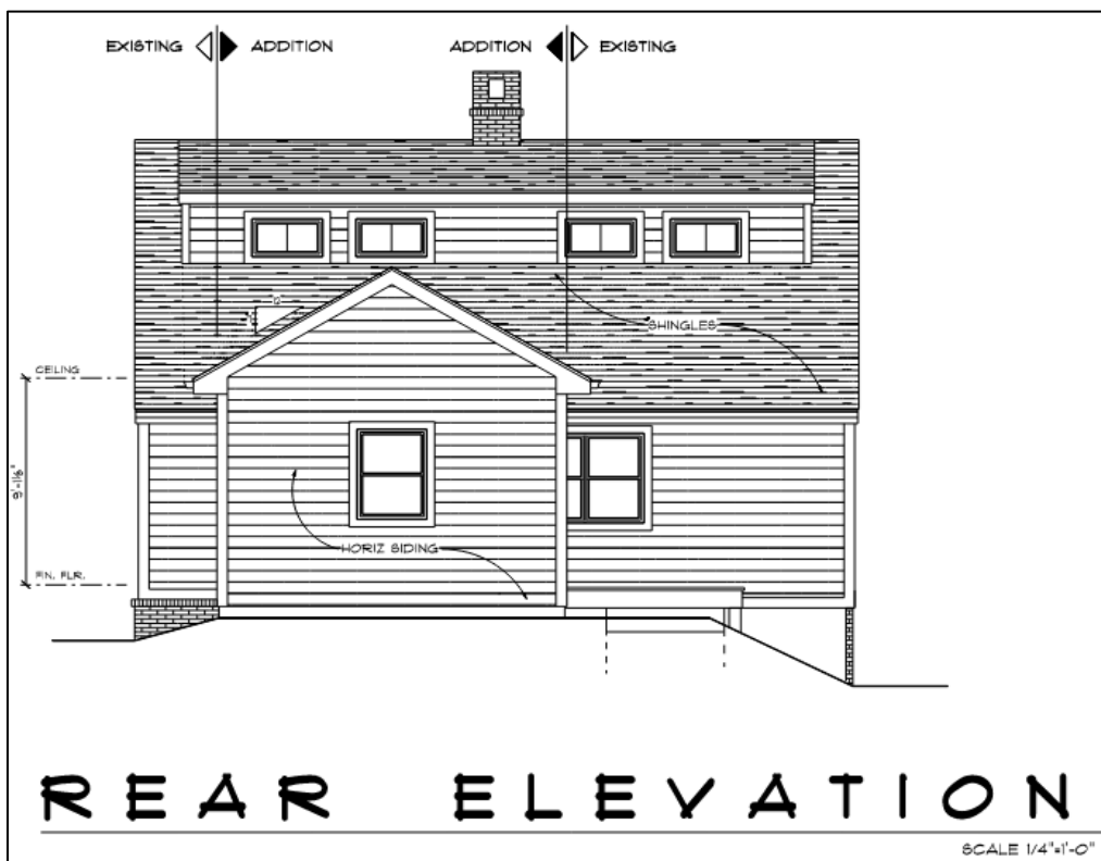
Figure 4: South elevation showcasing rear addition, deck, and shed dormers.
