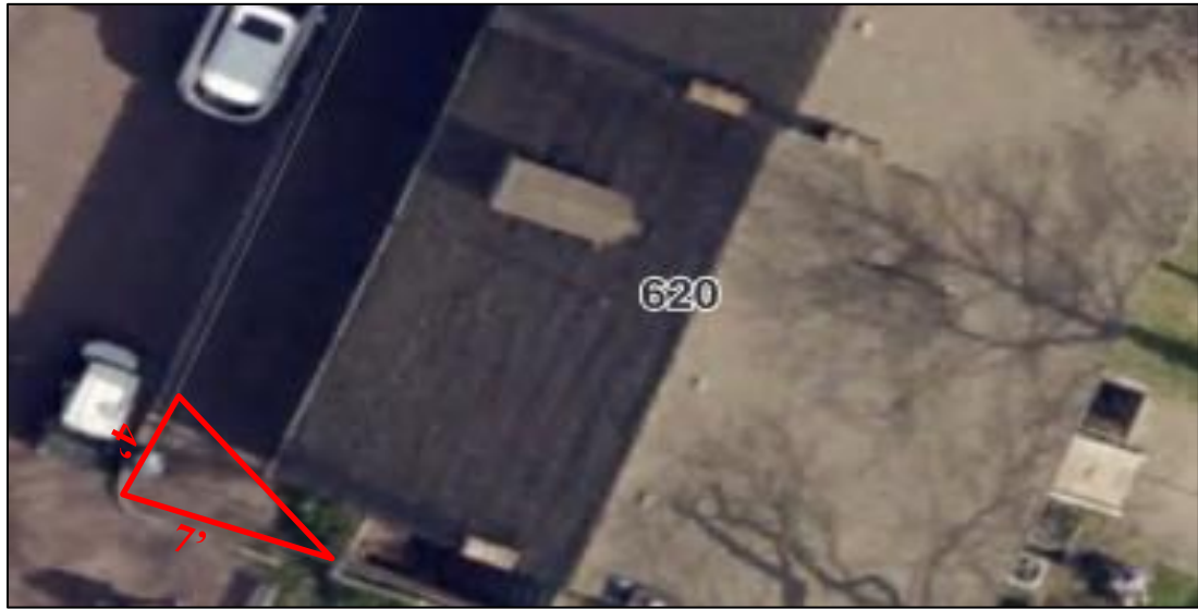
Figure 4: 620 S Main, with the non-compliant sight distance triangle identified.
