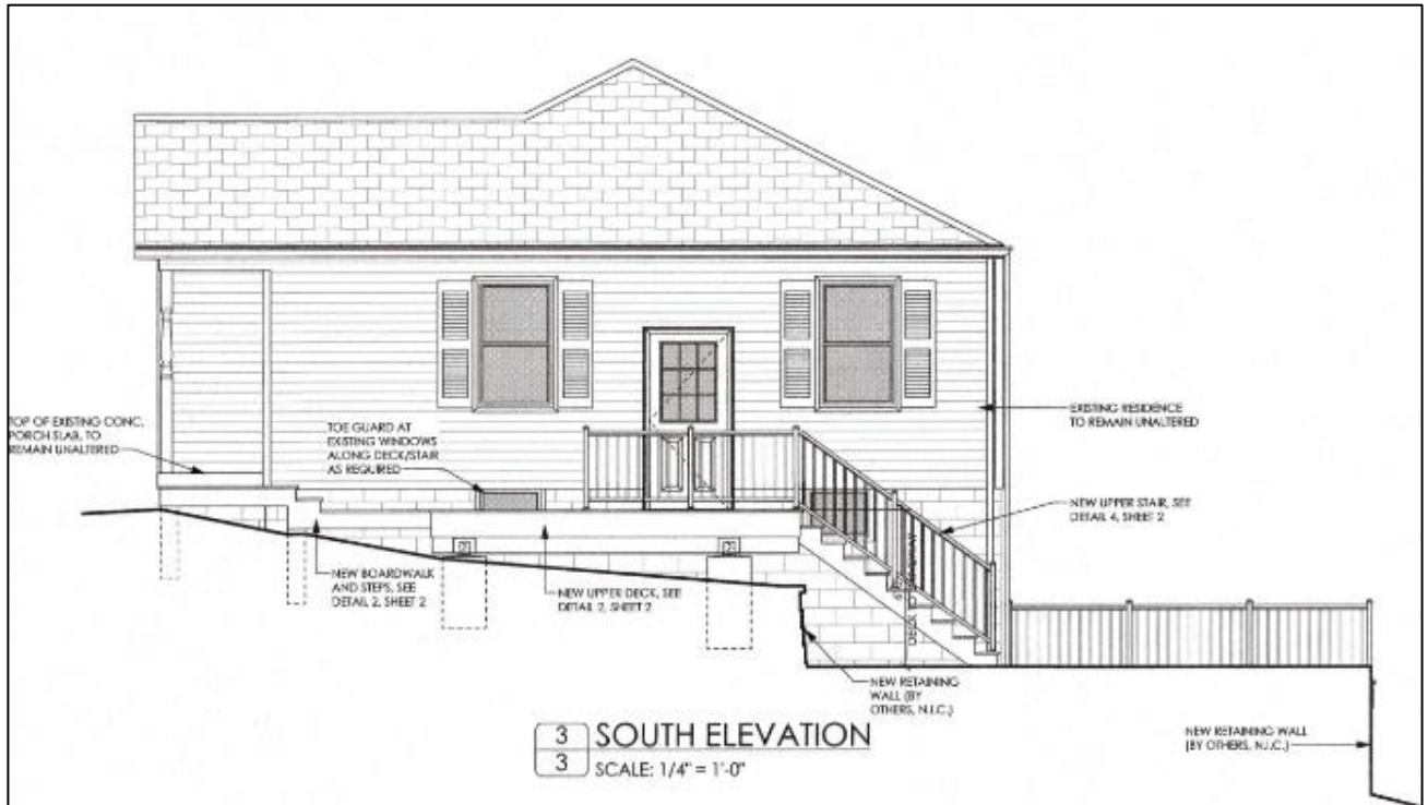
Figure 2: South Elevation showcasing proposed decks and stairs.
