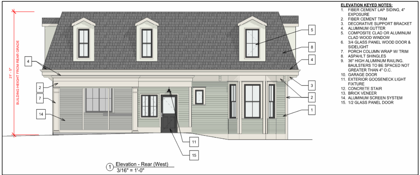
Figure 8: Rear-elevation of proposed new dwelling.
