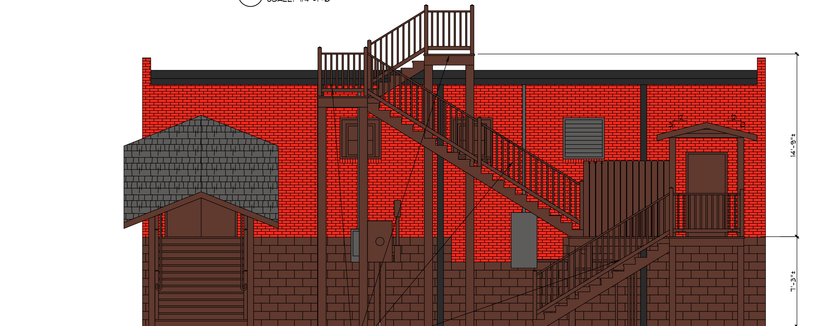
NEW EGRESS STAIRS TO GRADE FROM 2ND FLOOR ROOF w/ 42" WD GUARDRAIL, AND 36" HANDRAIL, PAINT TO MATCH EXISTING
