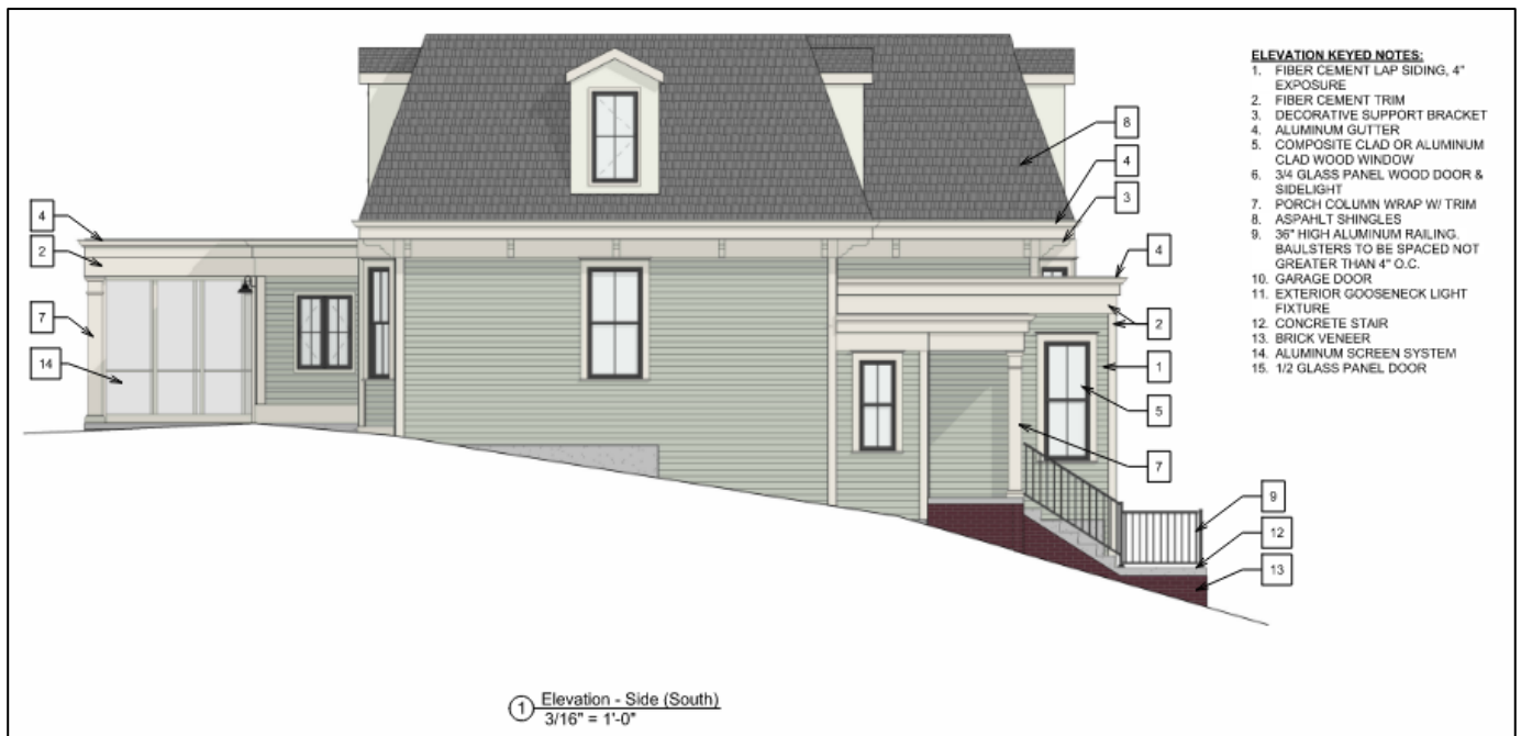
Figure 7: South-side elevation of proposed new dwelling.
