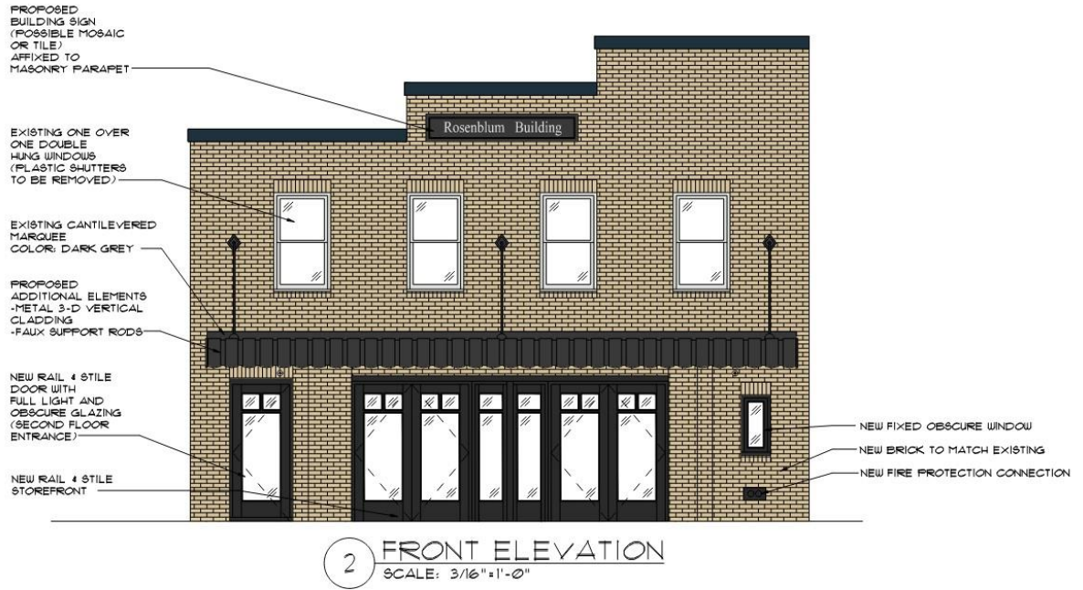
Figure 3: Elevation for proposed storefront alterations.
