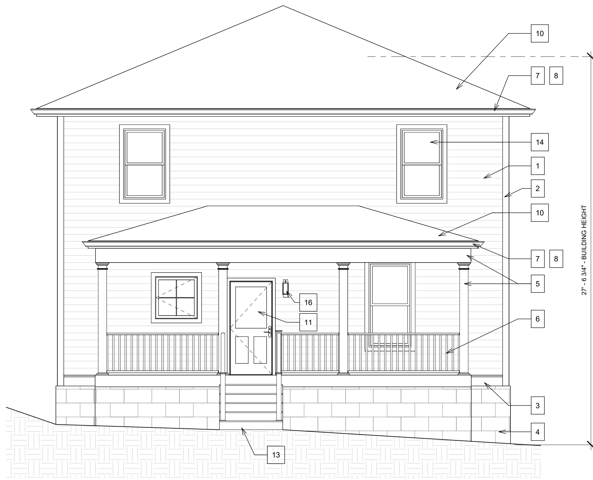
② Elevation - Front (South) 1/4" = 1'-0"
