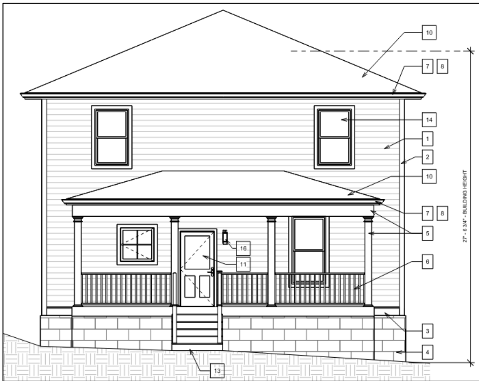
Figure 1: Front (south) elevation of the proposed new home.
