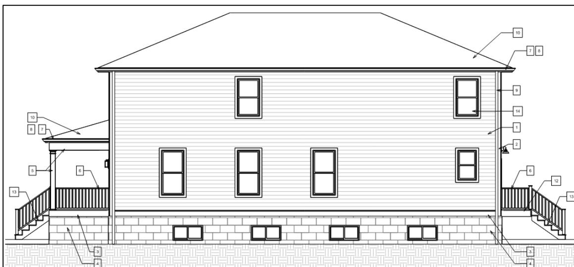
Figure 2: East side elevation of the proposed home.
